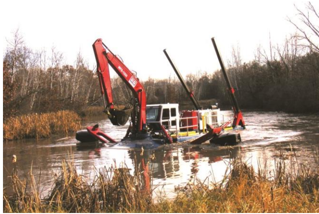
Figure 3.13. Floating amphibious excavator dredger. Suitable for shallow applications that need to dig into a liquid environment where a traditional excavator cannot work because of the inconsistent substrate. Photo credit: B. R. T. Impianti.
