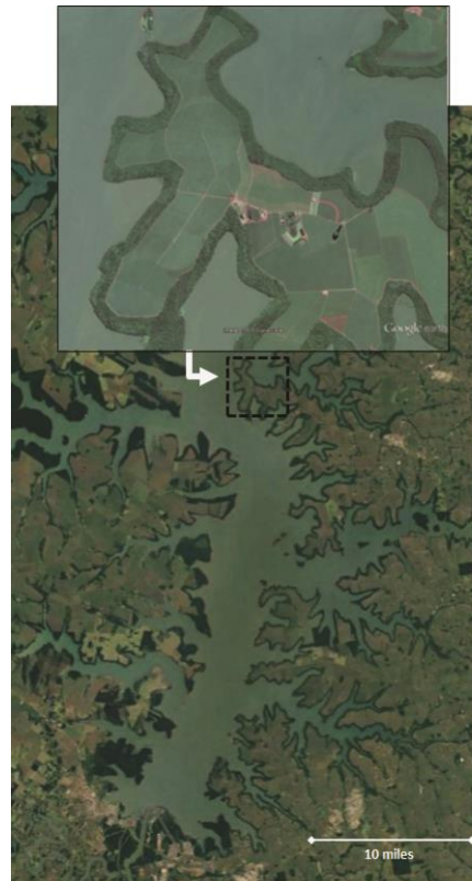
Figure 8.2. Itaipu Reservoir on the border of Paraguay (left) and Brazil (right). Note the well-developed managed forested riparian zone on the Brazilian side. The riparian zone is a minimum of 500 ft wide. Image credit: Google Earth.
