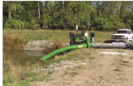
Figure 9.8. Portable pump used in Lake Odessa, Pools 17-18, Upper Mississippi River. Photo credit: USACE, Rock Island District.
