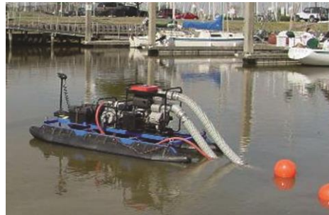
Figure 3.15. Mini-dredge for small sediment removal jobs Photo credit: Piranha, Albuquerque, New Mexico.
