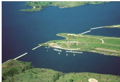
Figure 5.14. Jetties protecting large embayments in Branched Oak Reservoir, Nebraska. Photo credit: Nebraska Game and Parks Commission, Lincoln.
