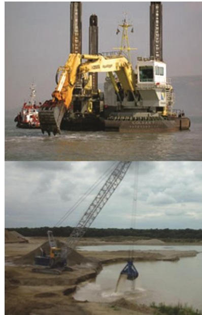
Figure 3.11. Backhoe (top) and clamshell (bottom) mechanical dredges. Photo credit: Dredge Source, Kansas City.
