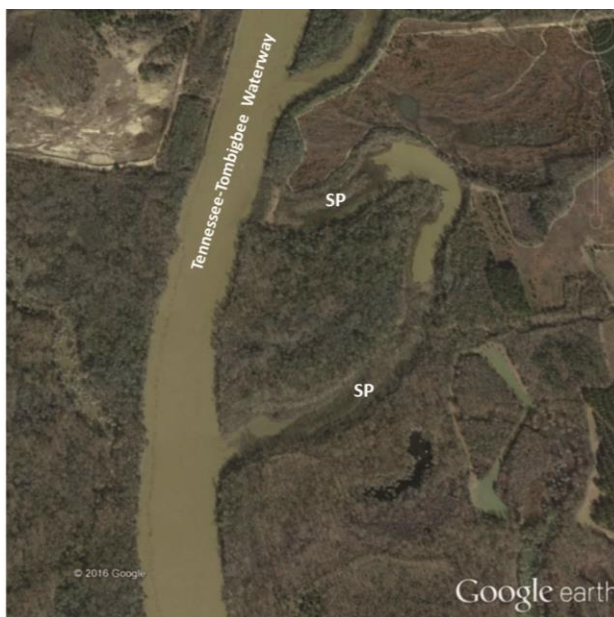
Figure 9.2. Bendway (channel of the original river) isolated from the uptake section of Columbus Lake reservoir, Mississippi. The river was channelized to facilitate navigation, and bendways were cut off on both sides of the new navigation channel. Cutoff bendways trap sediment that creates sediment plugs (SP) near their entrance and eventually become seasonally or permanently isolated from the reservoir unless weirs are installed to increase flow through the bendway or closing structures prevent flow into the bendway. Photo credit: Google Earth.
