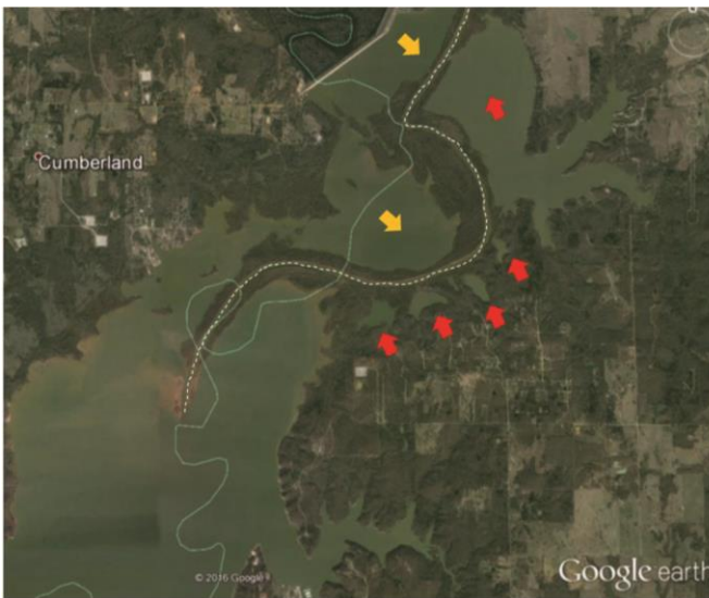
Figure 9.1. Lake Texoma, Oklahoma, where the Washita River feeds into the reservoir. The pale green line indicates the original river. The red arrows indicate areas that are nearly continually isolated from the main reservoir by sediment deposition and connect only at very high water levels. The yellow arrows indicate areas that are frequently isolated from the main reservoir. The dashed line indicates where inflow is depositing sediment following the pattern of natural river-levee deposition; these depositions are the ones primarily associated with isolation of areas and may be areas in which to target connectivity efforts. Photo credit: Google Earth; photograph annotated by T. Patton, Southeastern Oklahoma State University.
