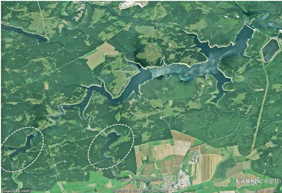
Figure 4.5. Rappbode Reservoir, Germany with two pre-dams (lower left corner). Photo credit: Google Earth.
