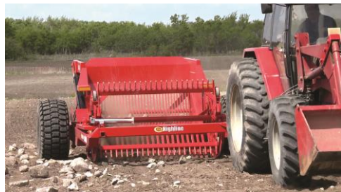
Figure 5.17. Rock often found scattered along the regulated zone can be collected with a rock picker and piled to construct stone reefs and/or shore reinforcements. Photo credit: Highline Manufacturing Ltd., Vonda, Saskatchewan.
