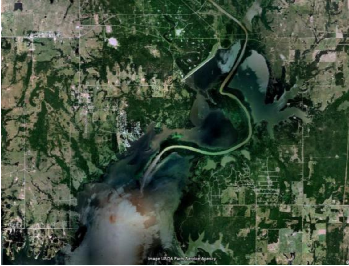
Figure 2.2 Satellite image of the Washita River arm of Lake Texoma, Texas-Oklahoma, showing extensive sediment deposition and channel formation.
